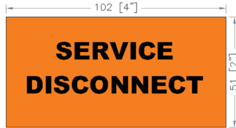
Figure-15 Service Disconnect Label
