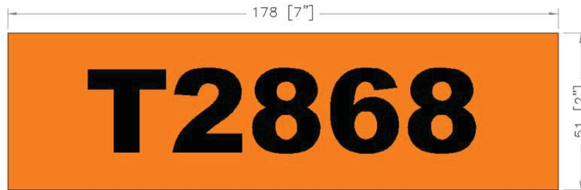
Figure-8 Transformer Identification Label (Example)
