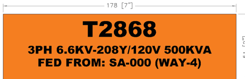
Figure-9 Transformer Information Label (Example)
